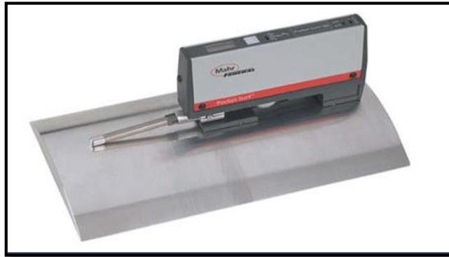
Figure(5):The Pocket Surf gauge.
