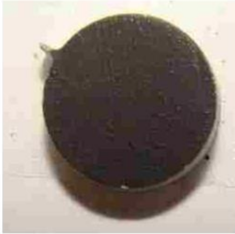
Figure 2-1: : Burn Epoxy Film Used to confirm testing and recording devices
